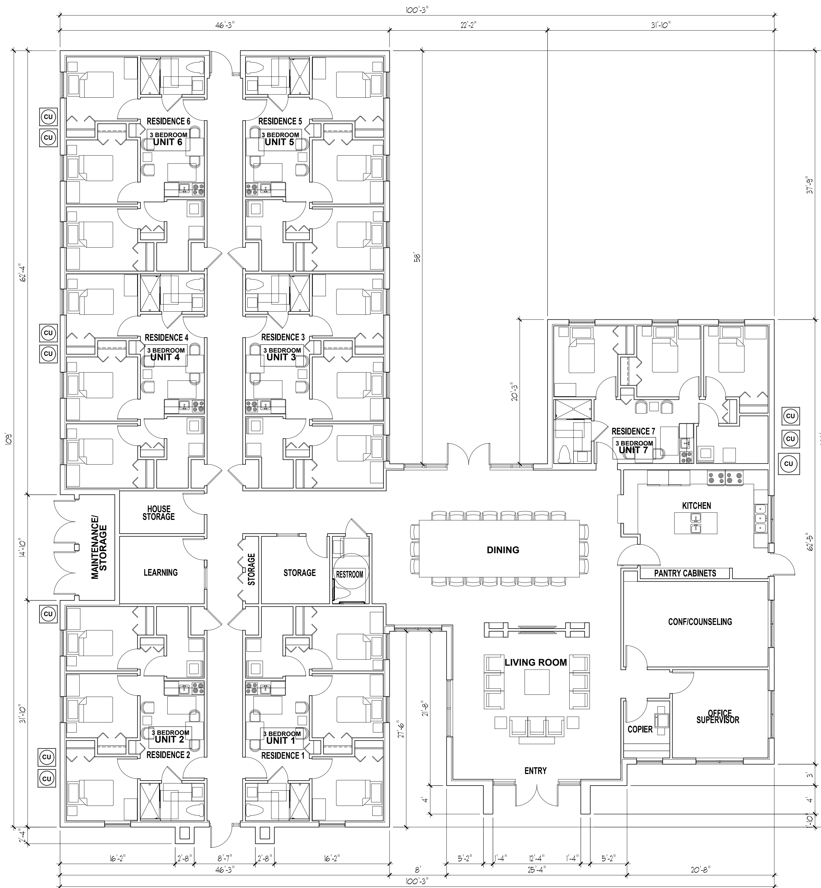
1 FLOOR PLAN SCALE: ONE INCH EQUALS 8 FEET
